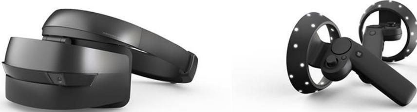
These Virtual Reality headsets have the benefit of using the spatial tracking software from the HoloLens, meaning there are no external lighthouses or sensors needed (as is the case with the HTC Vive and the Oculus Rift). They are very easy to setup and use and they interface to Demo3D using SteamVR in the same way other VR headsets do.
